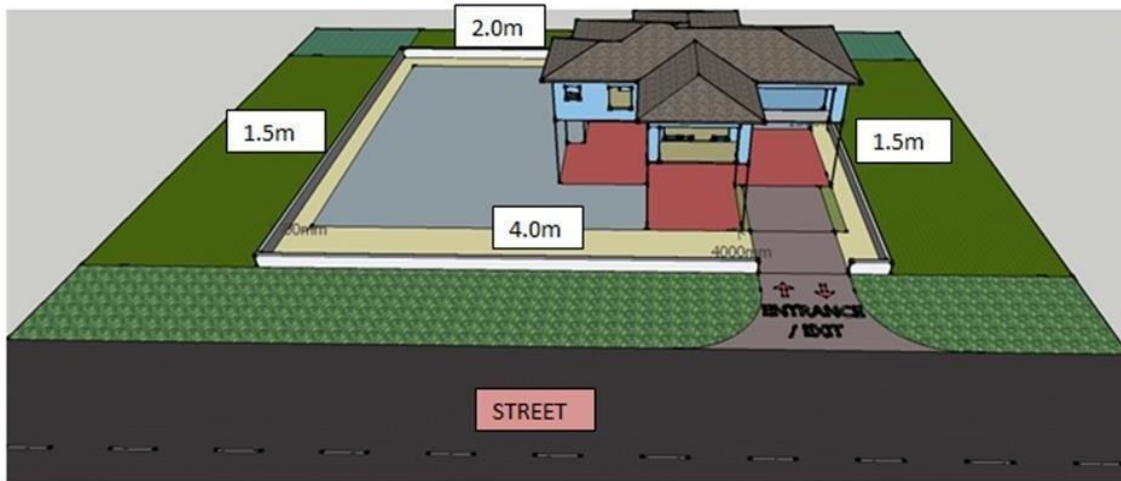
Diagram 1. Building lines on erf / Site abutting a street.
